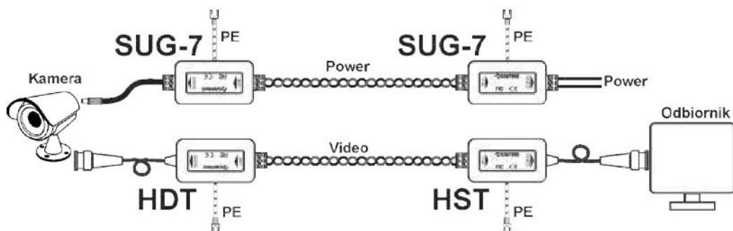
This model of the device should not be used for 24VAC alternating voltage, for example from network transformers.
