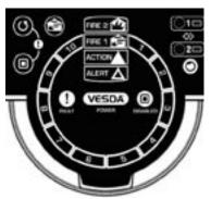
When the field service access door is open, the user has access to the RESET (), DISABLE Fire Test (), and Instant Fault Finder functions. When the Instant Fault Finder function is activated, the Smoke Dial converts to a fault indicator, with the dial segment numbers corresponding to the faults listed below.
